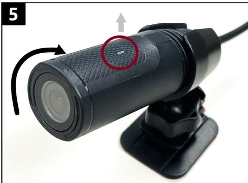
Rotate the camera so that the LED recording indicator faces upward.
