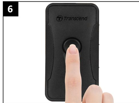
To power the camera on, long press the
